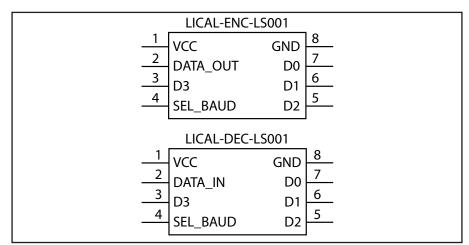
Figure 3: LS Series Encoder and Decoder Pin Assignments
