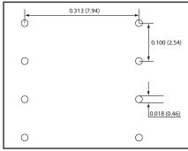
Figure 2: PCB Layout Dimensions
