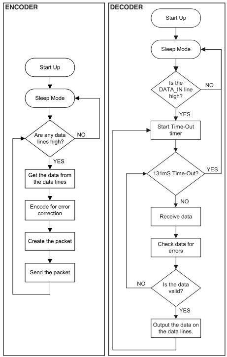
Figure 5: LS Series Encoder Flowchart
