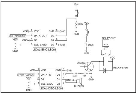
Figure 4: LS Series Application Circuits
