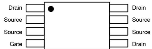
**Figure 2.** Pinouts for Single Die TSSOP
