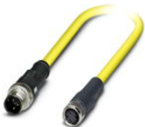
Sensor/Actuator cable, 3-position, PVC, yellow, Plug straight M12 SPEEDCON, A-coded, on Socket straight M8, Cable length: 1.5 m
