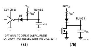
Figure 7. RUN/SS Pin Interfacing
