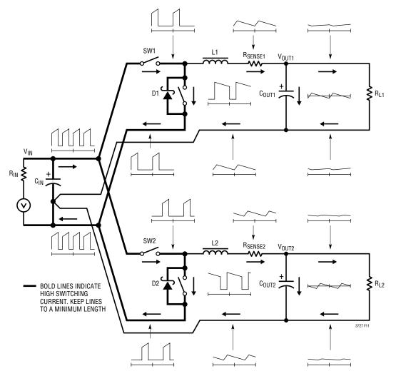
Figure 11. Branch Current Waveforms
