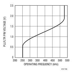
Figure 5. PLLFLTR Pin Voltage vs Frequency
