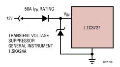
Figure 9. Automotive Application Protection
