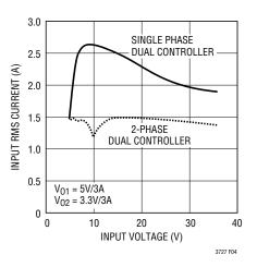
Figure 4. RMS Input Current Comparison
