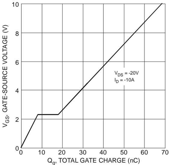
Figure 11 Gate-Charge Characteristics
