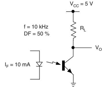
Fig. 14 - Switching Schematic
