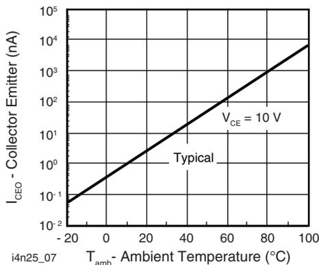
Fig. 7 - Collector Emitter Leakage Current vs. Temperature
