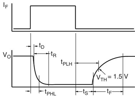
Fig. 13 - Switching Timing
