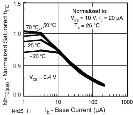
Fig. 11 - Normalized  $h_{FE}$  vs. Base Current and Temperature
