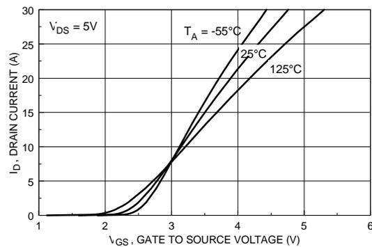
Figure 5. Transfer Characteristics.
