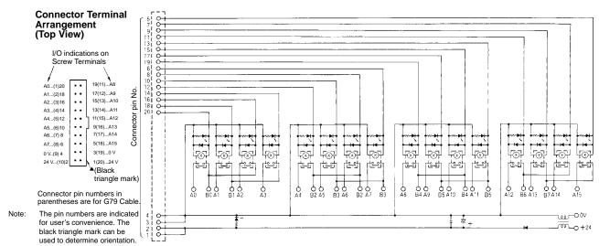
Note: Wiring shown above is for G6D Power Relays.
