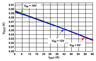
FIGURE 1. LOAD LINE REGULATION
