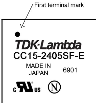
Marking: Followings are marked on the converter case
