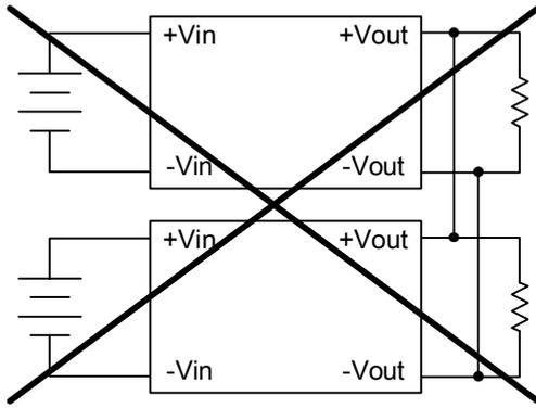
Fig.1 Parallel Connection
