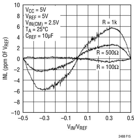
Figure 15. INL vs Differential Input Voltage and Reference Source Resistance for C<sub>REF</sub> > 1μF
