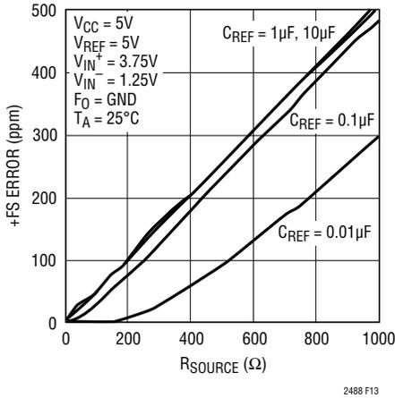
Figure 13. +FS Error vs R<sub>SOURCE</sub> at V<sub>REF</sub> (Large C<sub>REF</sub>)
