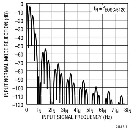
Figure 16. Input Normal Mode Rejection at DC
