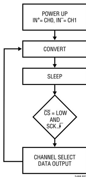
Figure 2. LTC2488 State Transition Diagram
