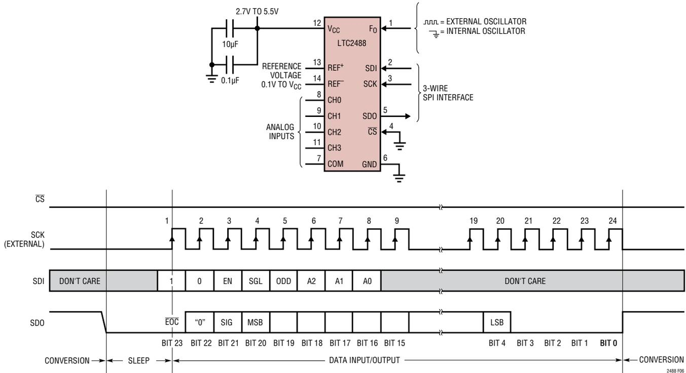
Figure 6. External Serial Clock, 3-Wire Operation ( $\overline{CS} = 0$ )
