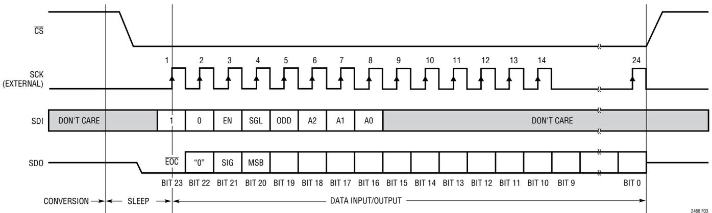
Figure 3. Channel Selection and Data Output Timing
