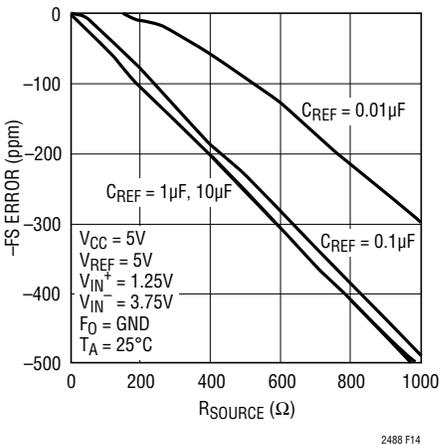
Figure 14. -FS Error vs R<sub>SOURCE</sub> at V<sub>REF</sub> (Large C<sub>REF</sub>)
