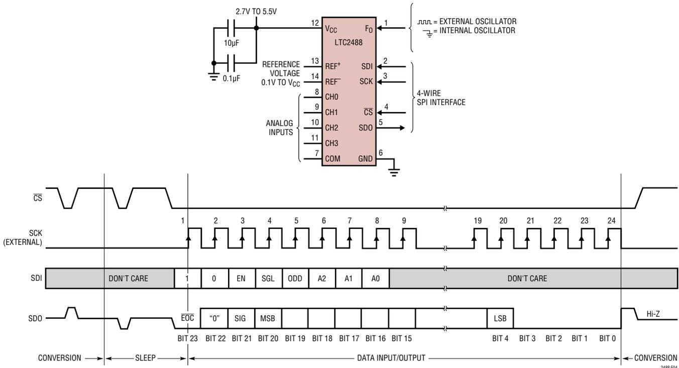
Figure 4. External Serial Clock, Single Cycle Operation
