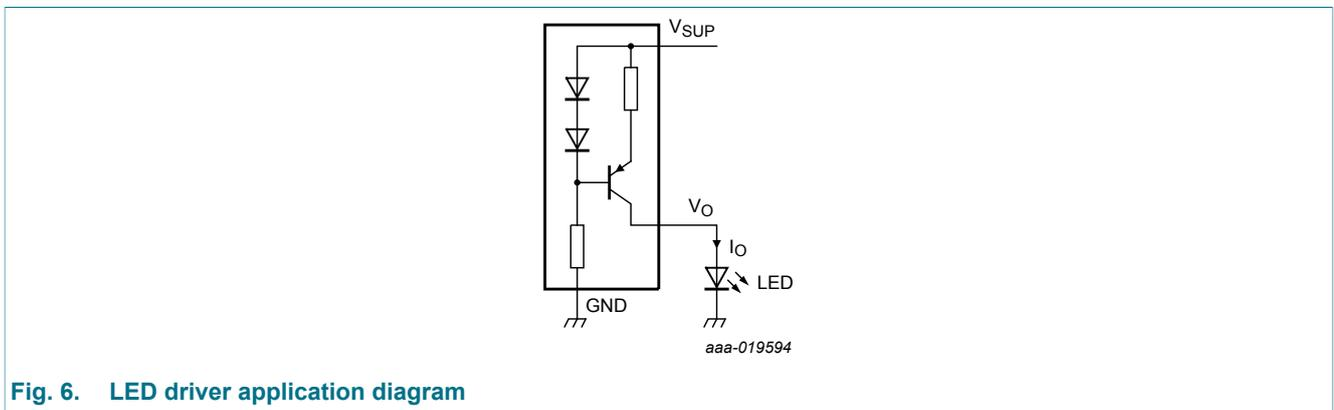
The output can be switched ON and OFF by connecting a Resistor-Equipped Transistor (RET), e.g. PDTC124XU; see Fig. 7
