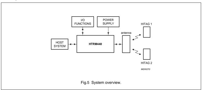
The HITAG proximity reader module HTRM440 (see Fig.5) is a part of a complete Radio Frequency Identification (RFID) system:
