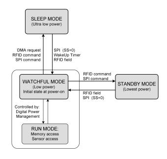
The Digital Controller can not exit this mode by itself. It can only exit it by an external interrupt: emission of a RFID field or asserting low the Slave Select input of the SPI (during a specified time)
