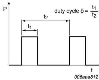
Fig. 16. Duty cycle definition
