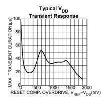
Figure 2b. Typical V<sub>DD</sub> Transient Response
