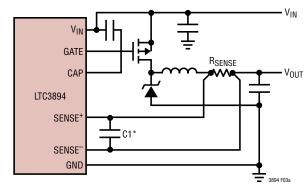
(3a) Using a Resistor to Sense Current
