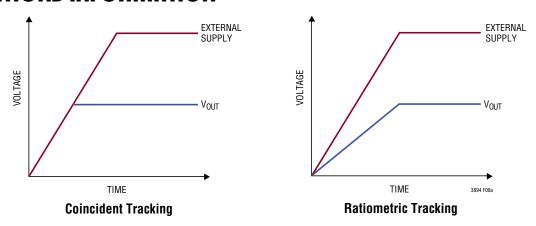
Figure 8(a). Two Different Modes of Output Tracking
