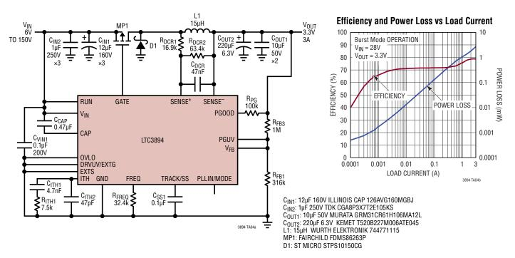
Figure 13. 6V to 150V Input, 3.3V/3A Output, 175kHz Step-Down Regulator
