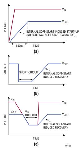
Figure 9. Internal Soft-Start (a) Allows Soft Start-Up without an External Soft-Start Capacitor and Allows Soft Recovery from (b) a Short-Circuit or (c) a V<sub>IN</sub> Dropout
