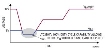
Figure 10. Typical Automotive Cold Crank
