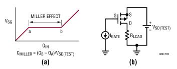
Figure 5. (a) Typical P-MOSFET Gate Charge Characteristics and (b) Test Set-Up to Generate Gate Charge Curve
