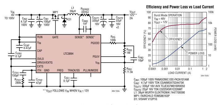
Figure 14. 6V to 100V Input, 12V/2A Output, 350kHz Step-Down Regulator
