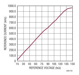
Figure 2. Switching Frequency vs Resistor on FREQ Pin
