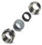
Metal screw connection up to 5 bar, thread length: 7 mm, cable diameter: 11 - 16 mm, WAF 27, screw connection: M25
