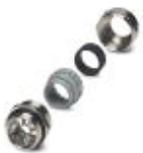
EMC screw connection up to 5 bar, thread length: 7.5 mm, cable diameter: 9.0 - 16.5 mm, WAF 29, screw connection: M25
