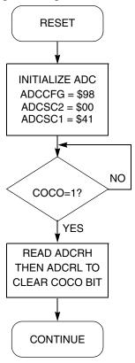
Figure 10-14. Initialization Flowchart Example
