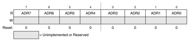
Figure 10-7. Data Result Low Register (ADCRL)
