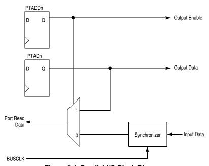
Figure 6-1. Parallel I/O Block Diagram
