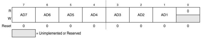
Figure 12-3. IIC Address Register (IICA)
