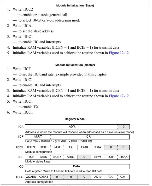
Figure 12-11. IIC Module Quick Start
