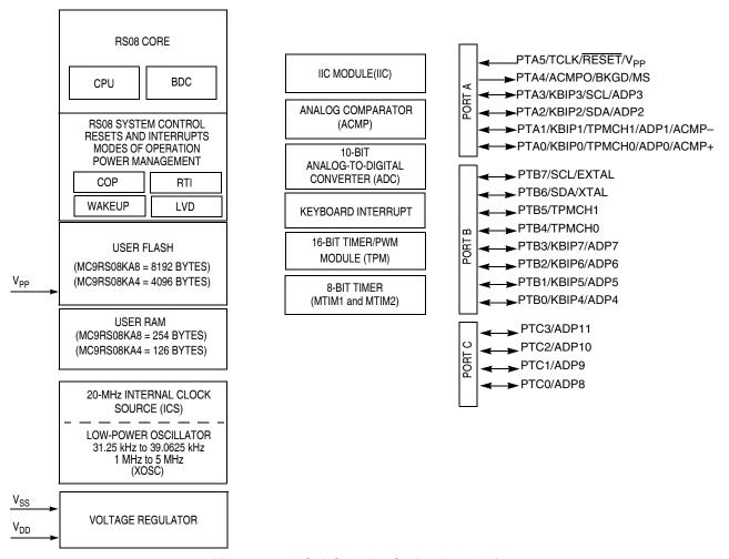
Figure 1-1. MC9RS08KA8 Series Block Diagram
