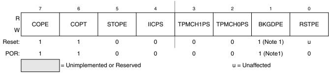
When the device is power on reset, BKGEPE is reset to 1. When the device is reset into normal operating mode (MS is high during reset), BKGDPE is reset to 1 if flash security is disengaged (SECD = 1). BKGDPE is reset to 0 if flash security is engaged (SECD = 0). When the device is reset into active BDM mode (MS is low during reset), BKGDPE is always reset to 1 such that BDM communication is allowed.
