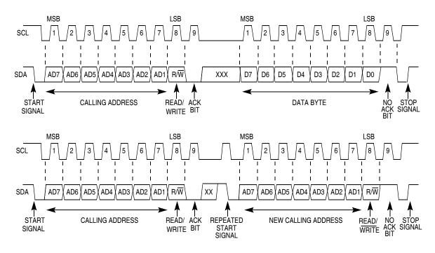
Figure 12-9. IIC Bus Transmission Signals
