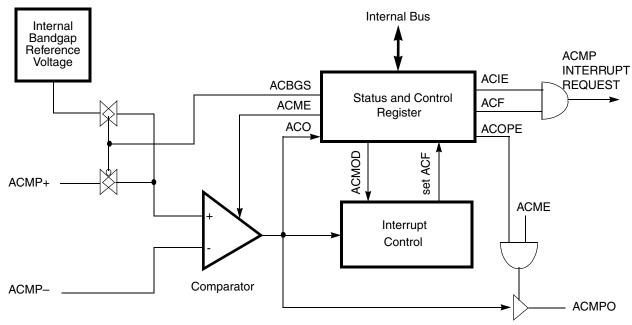
Figure 9-2. Analog Comparator (ACMP) Block Diagram
