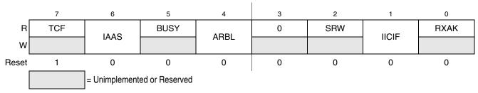
Figure 12-6. IIC Status Register (IICS)
