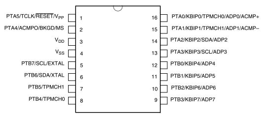
Figure 2-2. MC9RS08KA8 Series 16-Pin PDIP/SOIC/TSSOP Package
