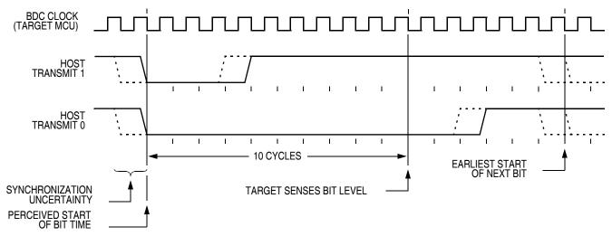
Figure 15-3. BDC Host-to-Target Serial Bit Timing
