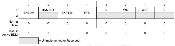
Figure 15-6. BDC Status and Control Register (BDCSCR)
