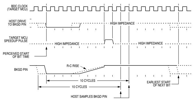
Figure 15-4. BDC Target-to-Host Serial Bit Timing (Logic 1)
