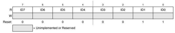
Figure 5-4. System Device Identification Register — Low (SDIDL)
