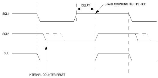
Figure 12-10. IIC Clock Synchronization
