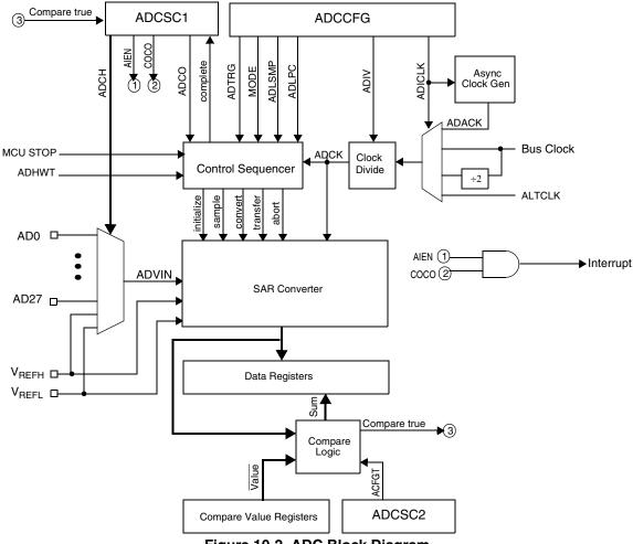
Figure 10-2. ADC Block Diagram
