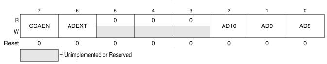
Figure 12-8. IIC Control Register (IICC2)
