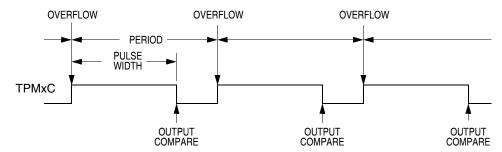
Figure 14-11. PWM Period and Pulse Width (ELSnA = 0)
