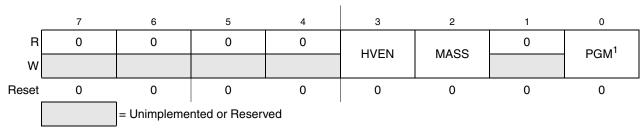
Figure 4-4. Flash Control Register (FLCR)
