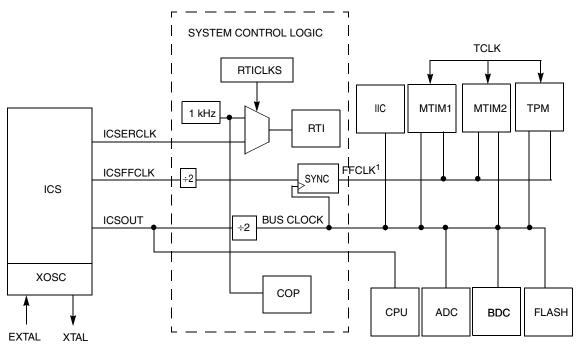
The fixed frequency clock (FFCLK) is internally synchronized to the bus clock and must not exceed one half of the bus clock frequency.
