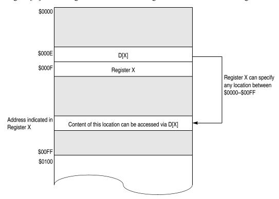
Figure 4-2. Indirect Addressing Registers
