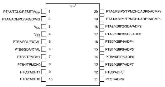
Figure 2-1. MC9RS08KA8 Series 20-Pin PDIP/SOIC Package
