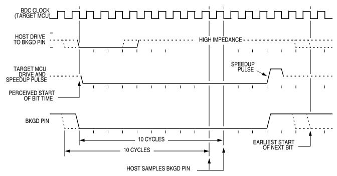
Figure 15-5. BDM Target-to-Host Serial Bit Timing (Logic 0)
