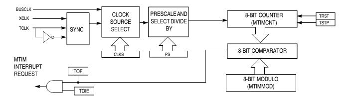
Figure 13-2. Modulo Timer (MTIM) Block Diagram
