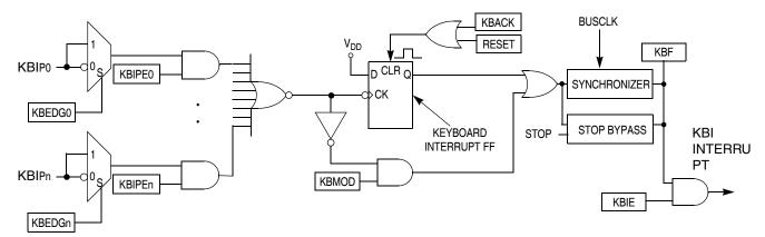
Figure 7-1. Keyboard Interrupt (KBI) Block Diagram
