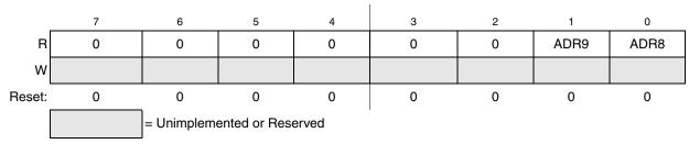
Figure 10-6. Data Result High Register (ADCRH)
