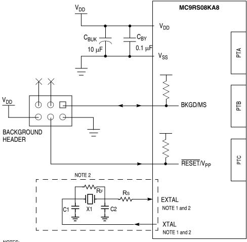
Figure 2-3. Reference System Connection Diagram
