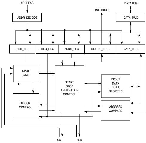
Figure 12-2. IIC Functional Block Diagram
