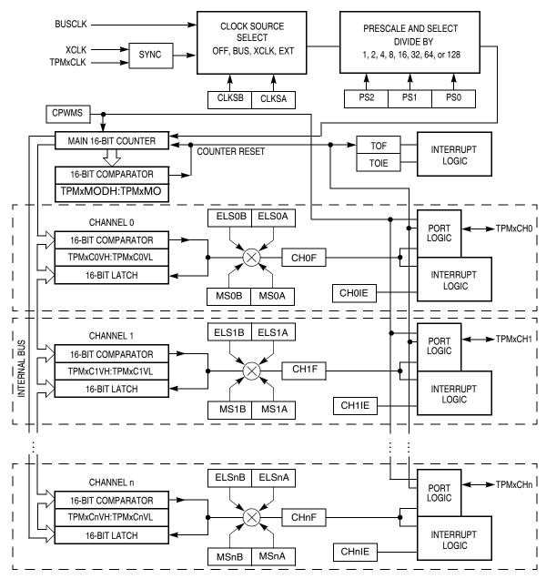
Figure 14-2. TPM Block Diagram
