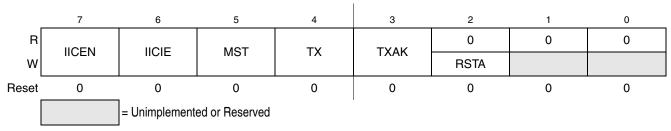
Figure 12-5. IIC Control Register (IICC1)
