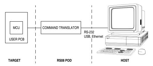
Figure 15-1. Connecting MCU to Host for Debugging
