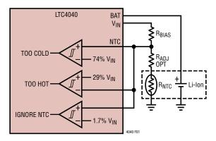
Figure 2. NTC Connections
