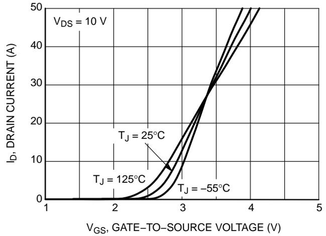
Figure 2. Transfer Characteristics
