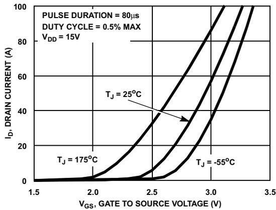
**Figure 7. Transfer Characteristics**
