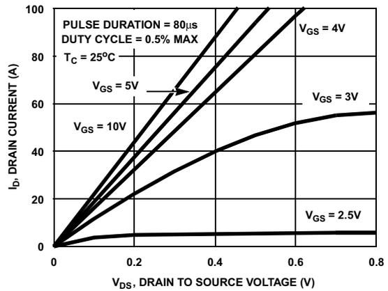
**Figure 8. Saturation Characteristics**
