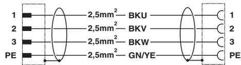
Contact assignment of M17 plugs/sockets
