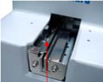
Loosen the set screw on the rail
