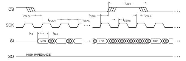
Figure 13-2. Serial Output Timing
