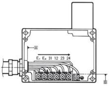
Tighten each wired terminal clockwise to a torque of 0.59 to 0.78  $N{\cdot}m.$
