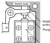
Rotating lever (with protruding part) Plunger (with groove)
