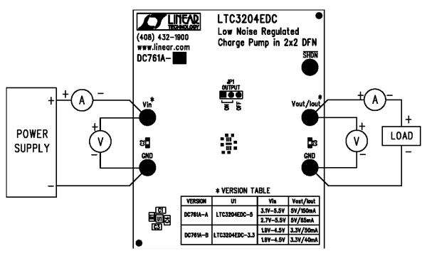
Figure 1. Proper Measurement Equipment Setup
