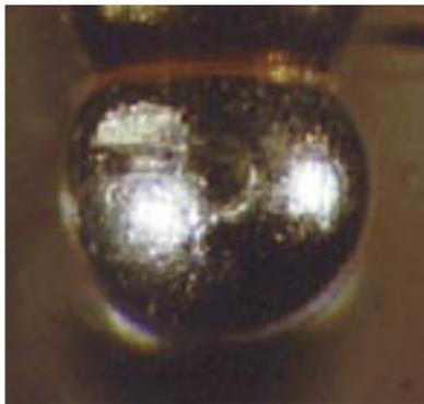
1.27 mm Solder Ball Deformation
