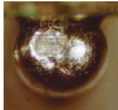
1.0 mm Solder Ball Deformation
