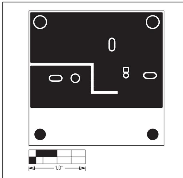
Figure 5. MAX5026 EV Kit PC Board Layout—Solder Side
