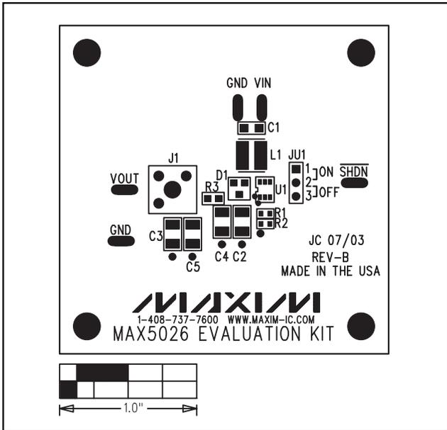
Figure 3. MAX5026 EV Kit Component Placement Guide—Top Silkscreen
