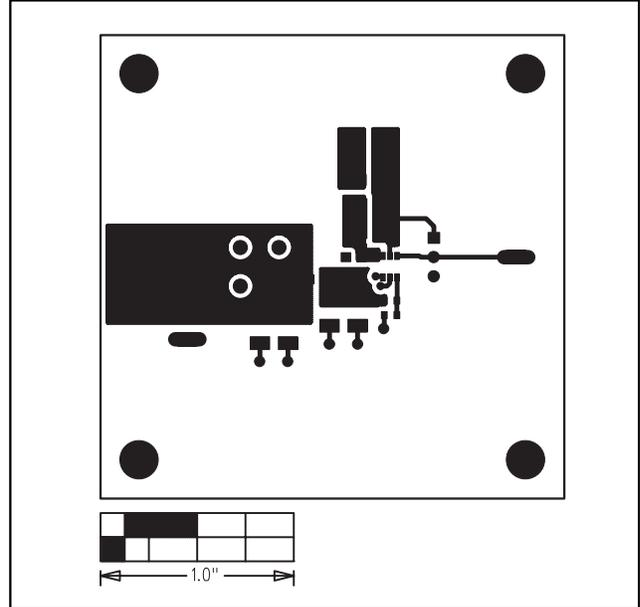
Figure 4. MAX5026 EV Kit PC Board Layout—Component Side
