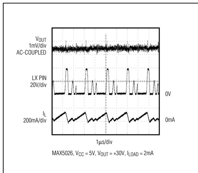
Figure 1. Medium-Load Switching Waveform with RC Filter
