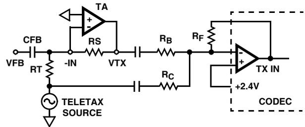
FIGURE 18. TELETAX SIGNALLING
