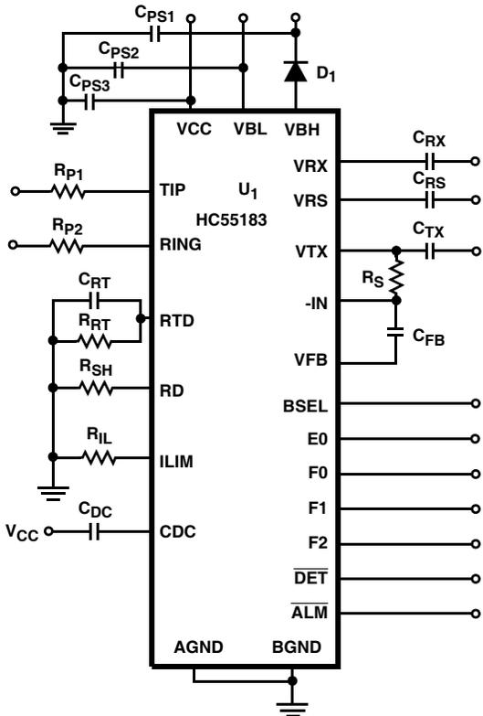
FIGURE 14. HC55183 BASIC APPLICATION CIRCUIT
