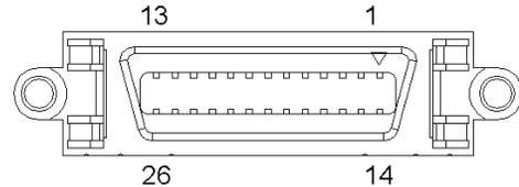
Figure 5: Connector CN3
