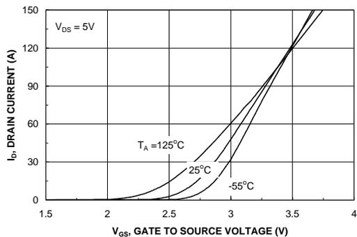
Figure 5. Transfer Characteristics.
