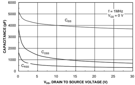
Figure 8. Capacitance Characteristics.
