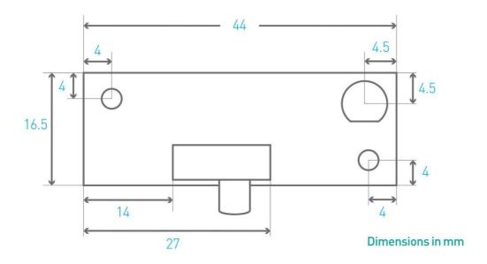
The 2 mounting holes are 3.3mm diameter.
