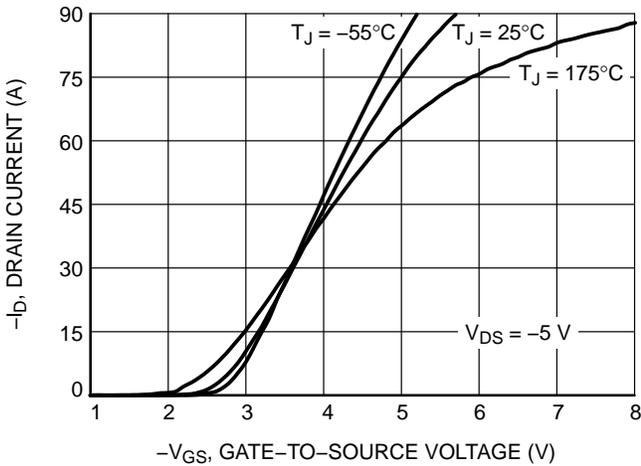
Figure 7. Transfer Characteristics
