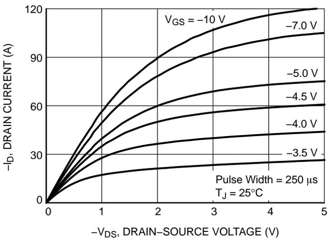
Figure 9. Saturation Characteristics
