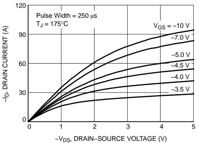
Figure 10. Saturation Characteristics
