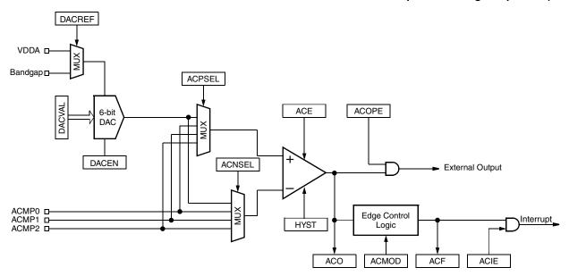
Figure 25-1. ACMP block diagram
