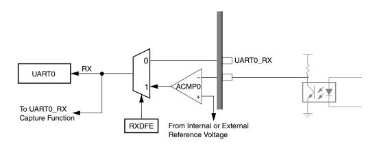
Figure 3-4. IR demodulation diagram
