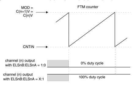
Figure 26-192. Channel (n) output if (C(n)V = C(n+1)V = MOD)
