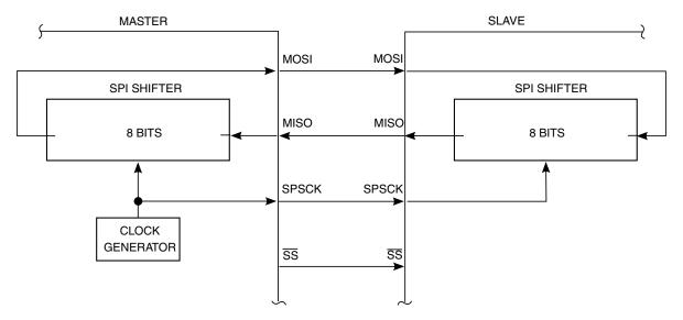
Figure 29-1. SPI system connections
