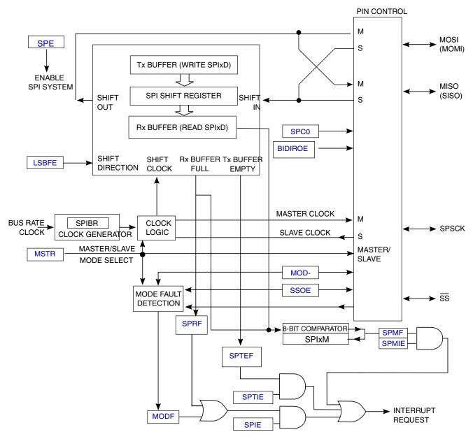
Figure 29-2. SPI module block diagram without FIFO
