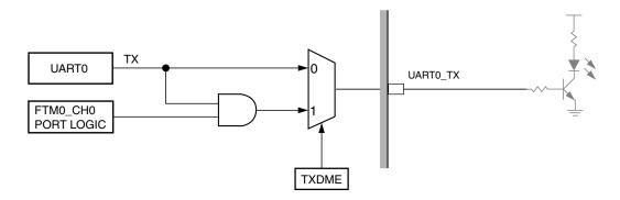
Figure 3-2. IR modulation diagram
