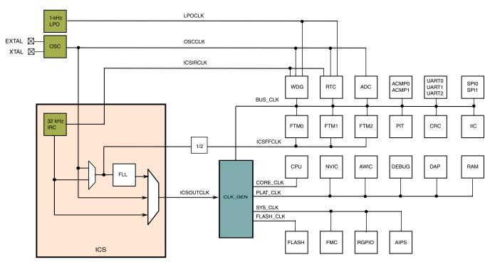
Figure 5-2. High-level clock distribution diagram
