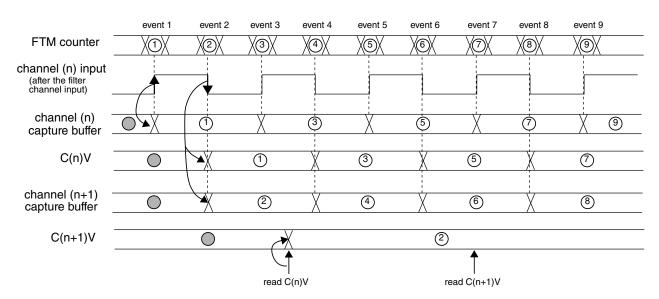
Figure 26-245. Dual Edge Capture mode read coherency mechanism
