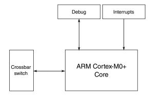
Figure 3-5. Core configuration
