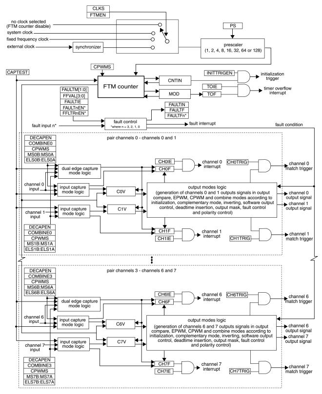
Figure 26-1. FTM block diagram
