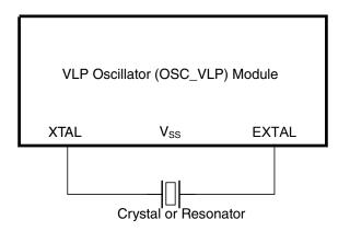
Figure 21-2. Crystal/resonator connections - connection 1
