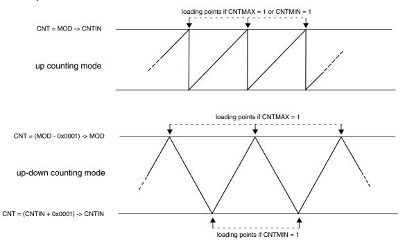
Figure 26-203. Boundary cycles and loading points
