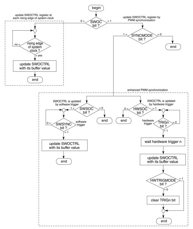
Figure 26-215. SWOCTRL register synchronization flowchart
