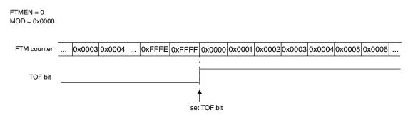
Figure 26-168. Example when the FTM counter is free running
