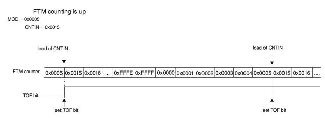
Figure 26-166. Example of up counting when the value of CNTIN is greater than the value of MOD
