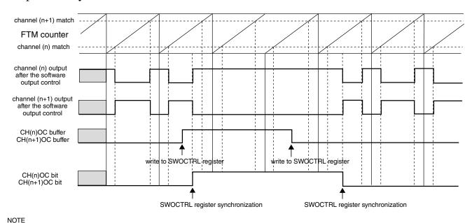
Figure 26-223. Example of software output control in Combine and Complementary mode
