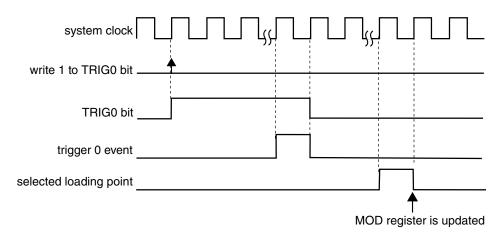
Figure 26-206. MOD synchronization with (SYNCMODE = 0), (HWTRIGMODE = 0), (PWMSYNC = 0), (REINIT = 0), and a hardware trigger was used
