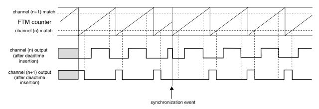
Figure 26-216. FTM counter synchronization
