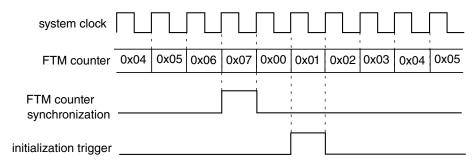
Figure 26-237. Initialization trigger is generated when there is the FTM counter synchronization
