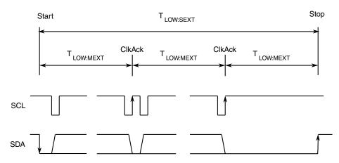
Figure 30-28. Timeout measurement intervals
