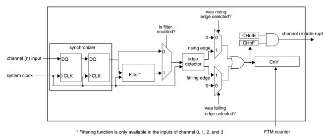
Figure 26-171. Input Capture mode
