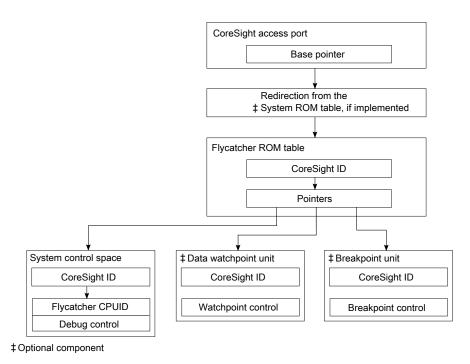
Figure 4-1. CoreSight discovery process
