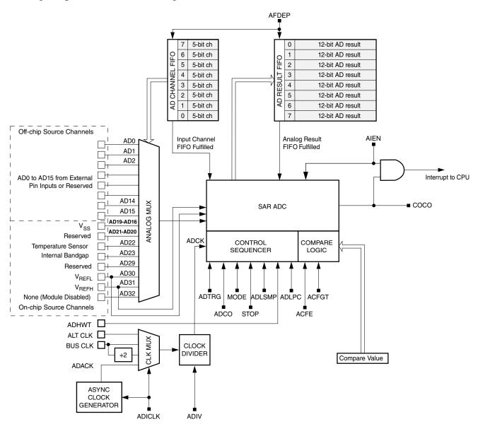
Figure 24-1. ADC Block Diagram
