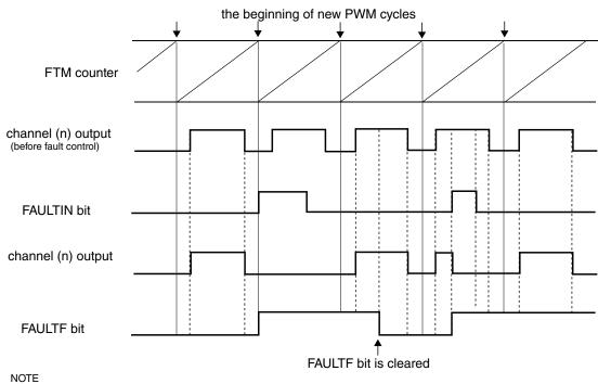
The channel (n) output is after the fault control with automatic fault clearing and POLn = 0.
