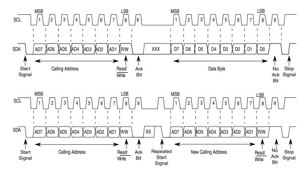
Figure 30-26. I2C bus transmission signals
