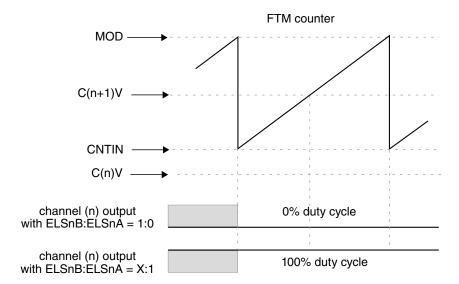
Figure 26-194. Channel (n) output if (C(n)V < CNTIN) and (CNTIN < C(n+1)V < MOD)
