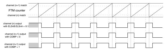
Figure 26-200. Channel (n+1) output in Complementary mode with (ELSnB:ELSnA = X:1)
