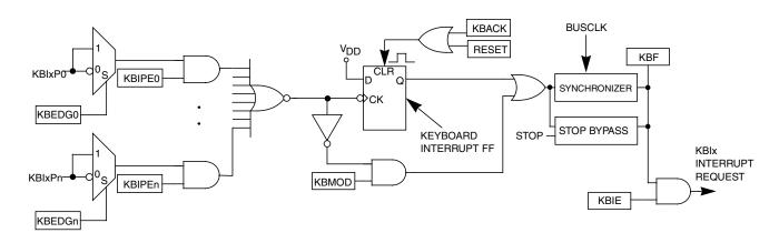
Figure 33-1. KBI block diagram
