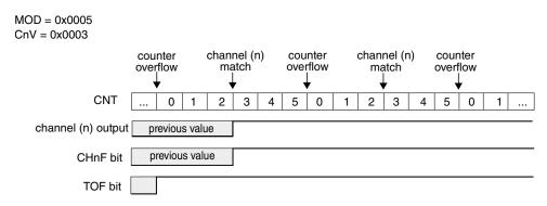
Figure 26-176. Example of the Output Compare mode when the match sets the channel output
