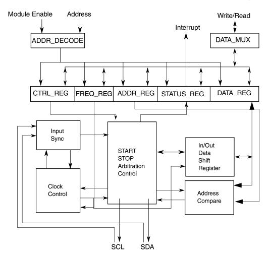
Figure 30-1. I2C Functional block diagram
