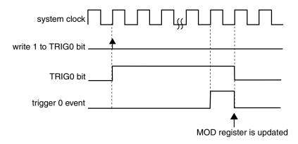
Figure 26-208. MOD synchronization with (SYNCMODE = 0), (HWTRIGMODE = 0), (PWMSYNC = 0), (REINIT = 1), and a hardware trigger was used
