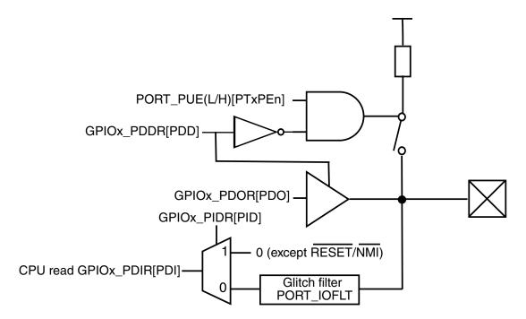
Figure 11-1. Normal I/O structure
