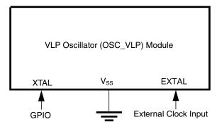
Figure 21-4. External clock connections
