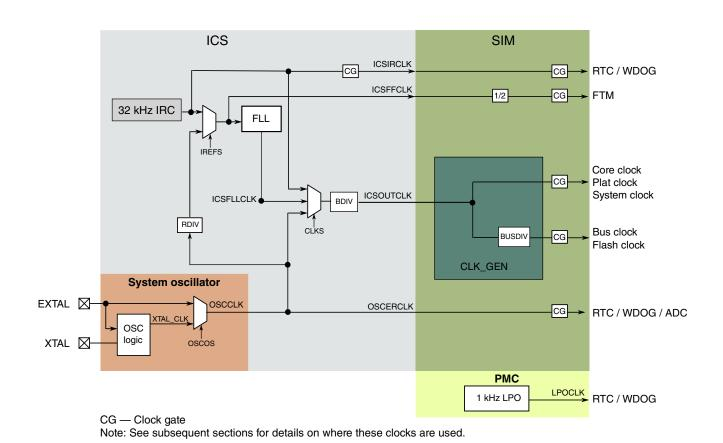
Figure 5-1. Clocking diagram
