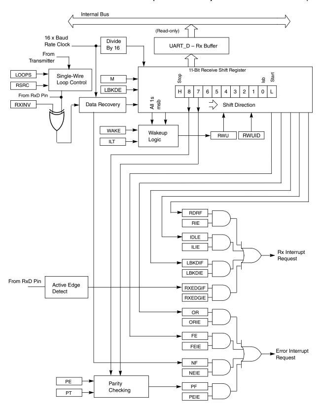
Figure 31-2. UART receiver block diagram
