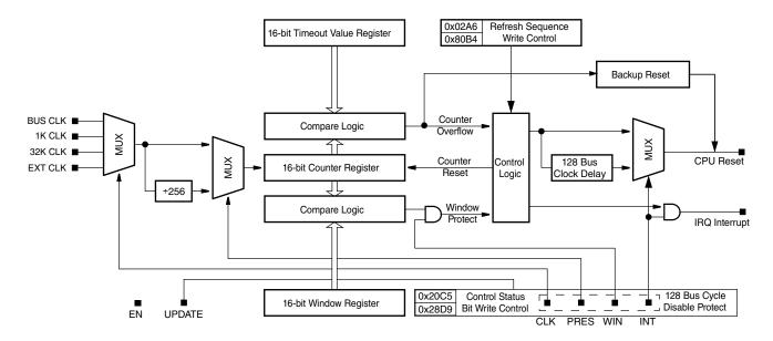
Figure 16-1. WDOG block diagram
