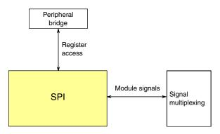
Figure 3-27. SPI configuration
