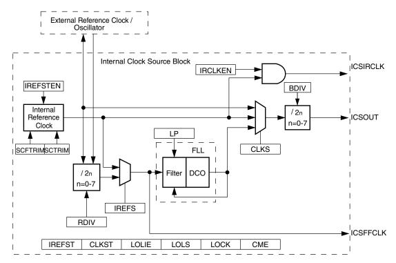
Figure 20-1. Internal clock source (ICS) block diagram
