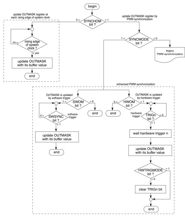
Figure 26-210. OUTMASK register synchronization flowchart
