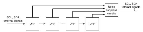
Figure 30-29. Programmable input glitch filter diagram
