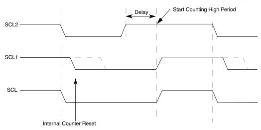
Figure 30-27. I2C clock synchronization
