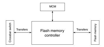
Figure 3-19. Flash memory controller configuration
