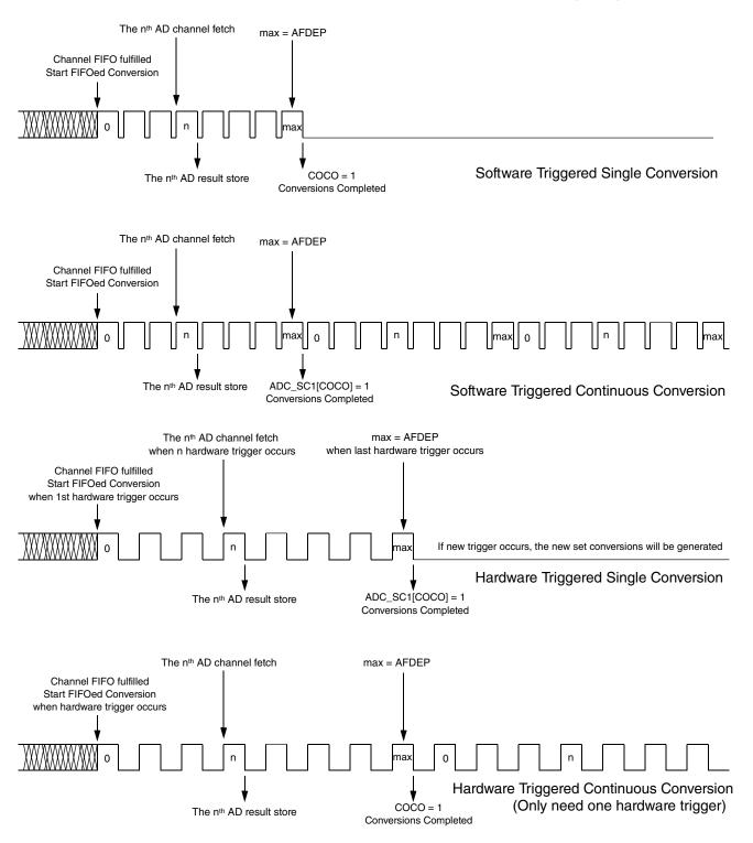
Figure 24-10. ADC FIFO conversion sequence
