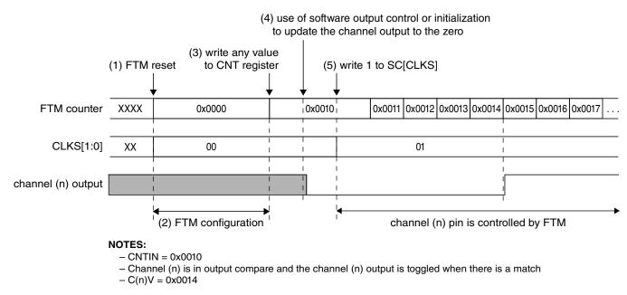
Figure 26-249. FTM behavior after reset when the channel (n) is in Output Compare mode
