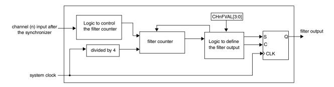
Figure 26-172. Channel input filter
