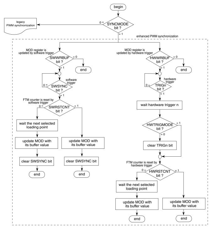
Figure 26-204. MOD register synchronization flowchart
