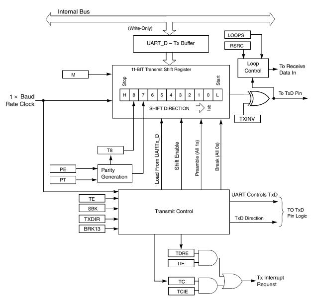
Figure 31-1. UART transmitter block diagram
