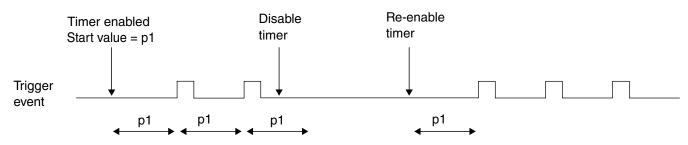
Figure 27-15. Stopping and starting a timer
