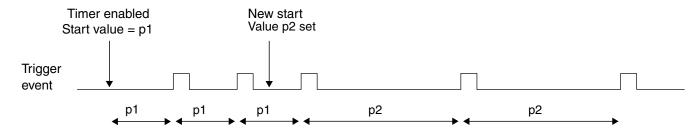
Figure 27-17. Dynamically setting a new load value
