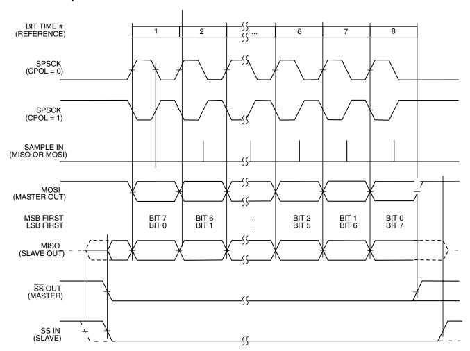
Figure 29-21. SPI clock formats (CPHA = 1)
