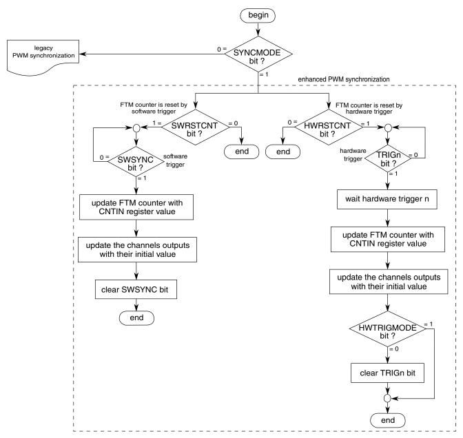
Figure 26-217. FTM counter synchronization flowchart
