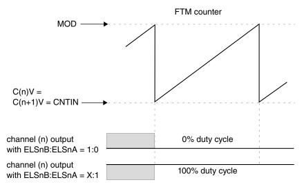
Figure 26-191. Channel (n) output if (C(n)V = C(n+1)V = CNTIN)
