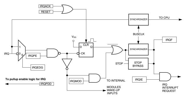
Figure 23-1. IRQ module block diagram
