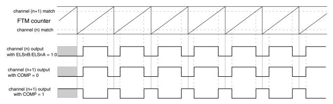
Figure 26-199. Channel (n+1) output in Complementary mode with (ELSnB:ELSnA = 1:0)
