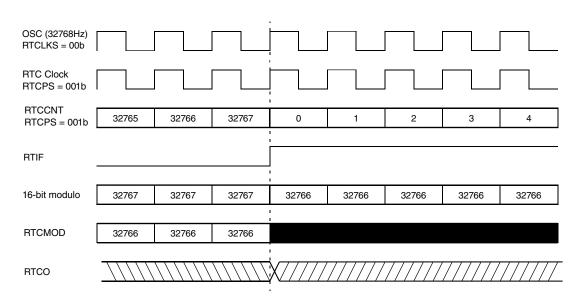
Figure 28-5. RTC counter overflow example
