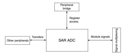
Figure 3-22. 12-bit SAR ADC configuration
