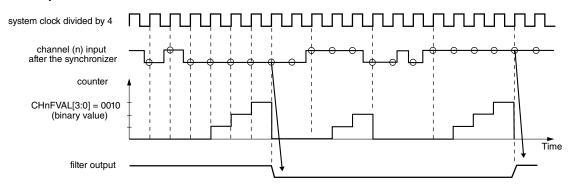
Figure 26-173. Channel input filter example
