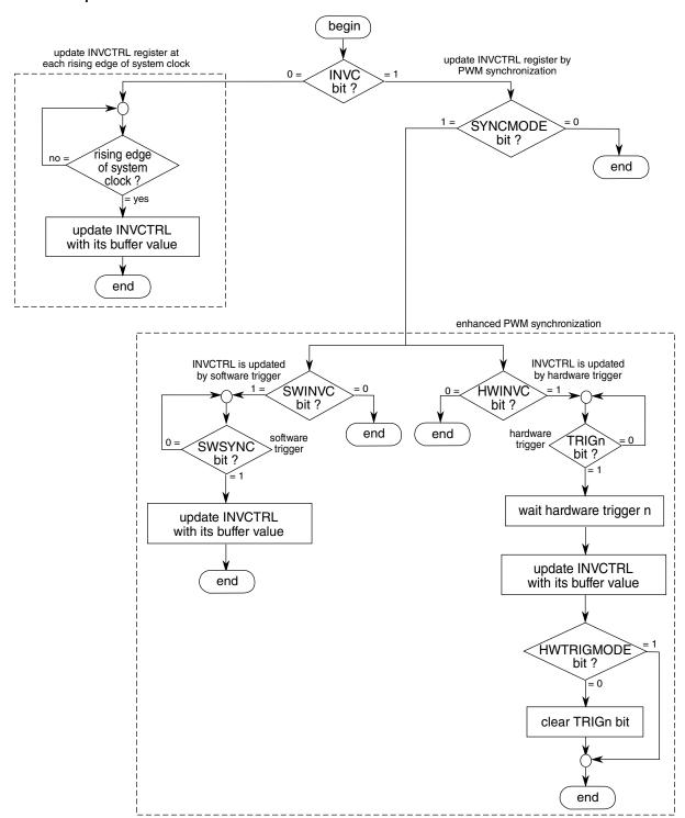
Figure 26-214. INVCTRL register synchronization flowchart
