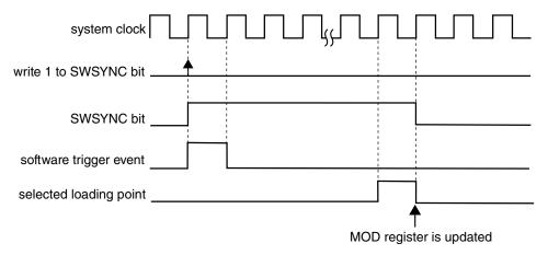
Figure 26-205. MOD synchronization with (SYNCMODE = 0), (PWMSYNC = 0), (REINIT = 0), and software trigger was used
