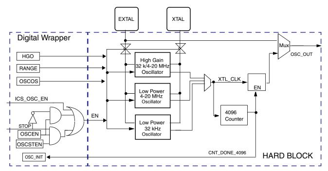
Figure 21-1. OSC module block diagram
