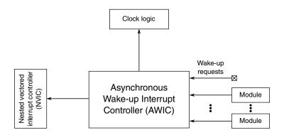
Figure 3-7. Asynchronous wake-up interrupt controller configuration
