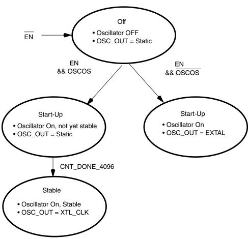
Figure 21-6. OSC module state diagram
