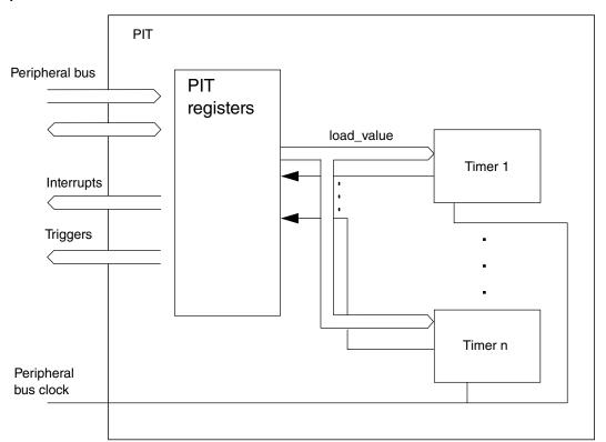
Figure 27-1. Block diagram of the PIT
