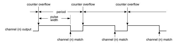
Figure 26-177. EPWM period and pulse width with ELSnB:ELSnA = 1:0
