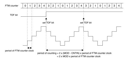
Figure 26-167. Example of up-down counting when CNTIN = 0x0000
