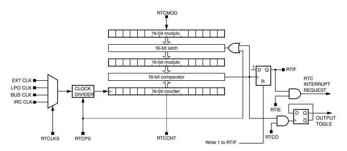
Figure 28-1. Real-time counter (RTC) block diagram
