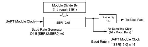
Figure 31-35. UART baud rate generation
