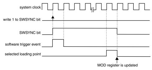
Figure 26-209. MOD synchronization with (SYNCMODE = 0) and (PWMSYNC = 1)
