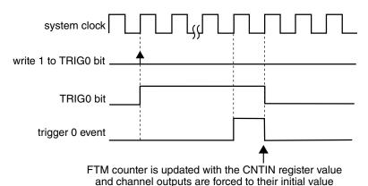
Figure 26-220. FTM counter synchronization with (SYNCMODE = 0), (HWTRIGMODE = 0), (REINIT = 1), (PWMSYNC = 1), and a hardware trigger was used
