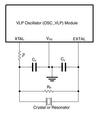
Figure 21-3. Crystal/resonator connections - connection 2
