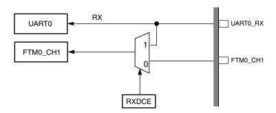
Figure 3-3. UARTO RX capture function diagram
