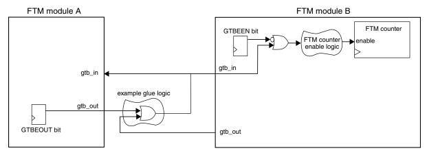
Figure 26-247. Global time base (GTB) block diagram
