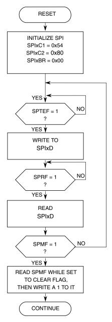
Figure 29-24. Initialization Flowchart Example for SPI Master Device
