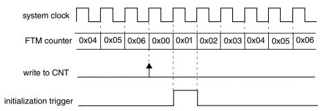
Figure 26-236. Initialization trigger is generated when there is a write to CNT register
