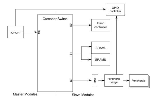
Figure 3-11. Crossbar-Light switch integration
