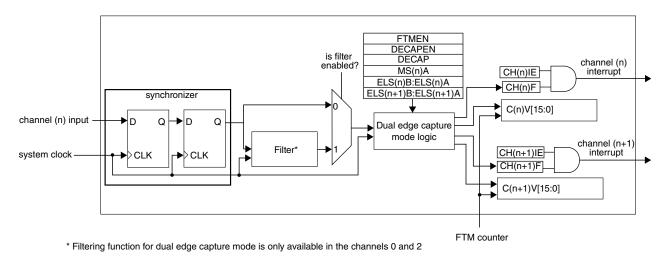
Figure 26-240. Dual Edge Capture mode block diagram
