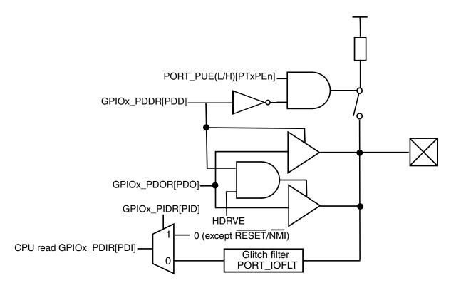
Figure 11-3. High drive I/O structure
