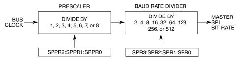
Figure 29-23. SPI baud rate generation
