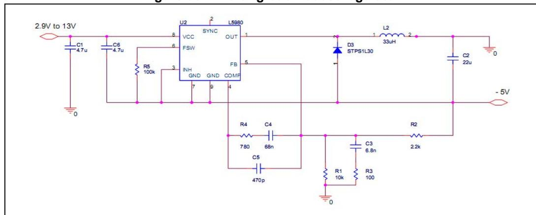
The GND pin of the device is connected to the output voltage so, given the output voltage, input voltage range is limited by the maximum voltage the device can withstand across VCC and GND (18 V). Thus if the output is -5 V the input voltage can range from 2.9 V to 13 V.
