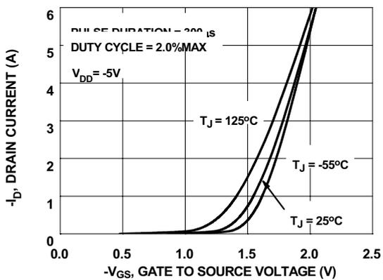
**Figure 5. Transfer Characteristics**
