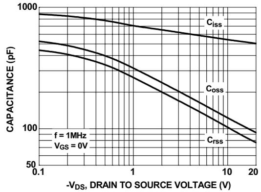
**Figure 8. Capacitance Characteristics**
