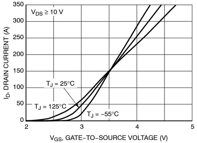
Figure 2. Transfer Characteristics
