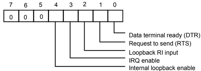
Bit 4: When this bit is set to a logical 1, the UART enters diagnostic mode by an internal loopback, as follows:
