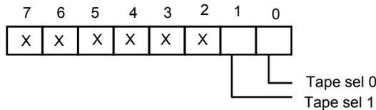
If three mode FDD function is enabled (EN3MODE = 1 in CR9), the bit definitions are as follows:
