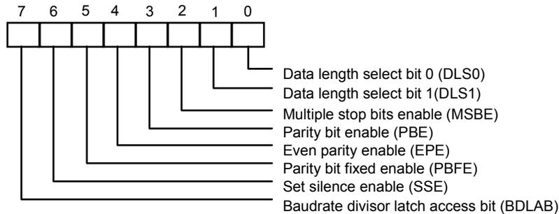
Bit 7: BDLAB. When this bit is set to a logical 1, designers can access the divisor (in 16-bit binary format) from the divisor latches of the baudrate generator during a read or write operation. When this bit is reset, the Receiver Buffer Register, the Transmitter Buffer Register, or the Interrupt Control Register can be accessed.
