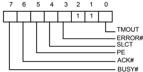
Bit 7: This signal is active during data entry, when the printer is off-line during printing, when the print head is changing position, or during an error state. When this signal is active, the printer is busy and cannot accept data.
