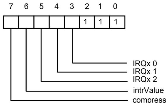
Bit 7: This bit is read-only. It is at low level during a read. This means that this chip does not support hardware RLE compression.
