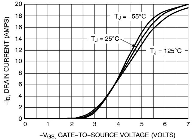
**Figure 2. Transfer Characteristics**
