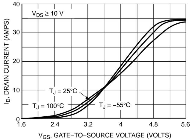
Figure 2. Transfer Characteristics
