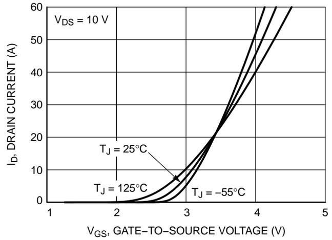
Figure 2. Transfer Characteristics
