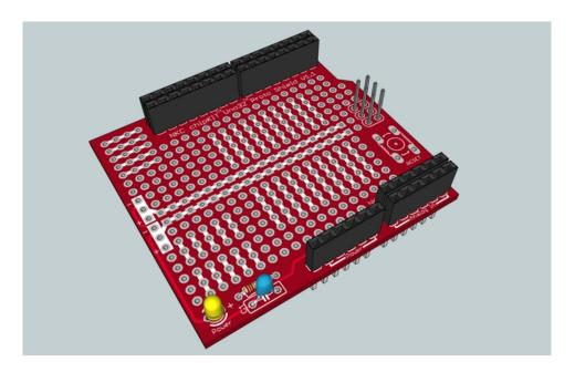
The RESET switch is necessary if you want to reset the chipKIT Uno32 board from the top
