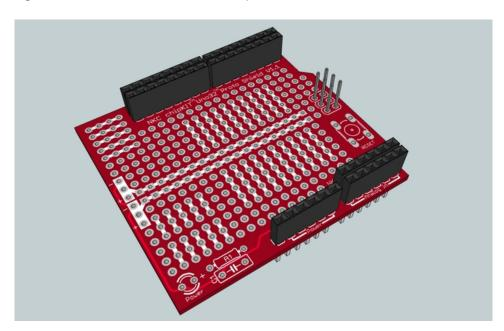
The LED with the associated resistor and filtering capacitor is to add a POWER indicator, meaning you have 5V power from the chipKIT Uno32 board to the ProtoShield.
