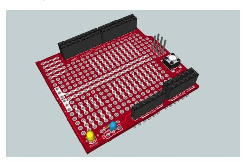
The little 6-pin male header with the 2 jumpers are used to configure how you want to use the 2 power BUSES in the middle of the board. You can send +5V to one of them, GND to the other, or +5 or GND to both of them at the same time.
