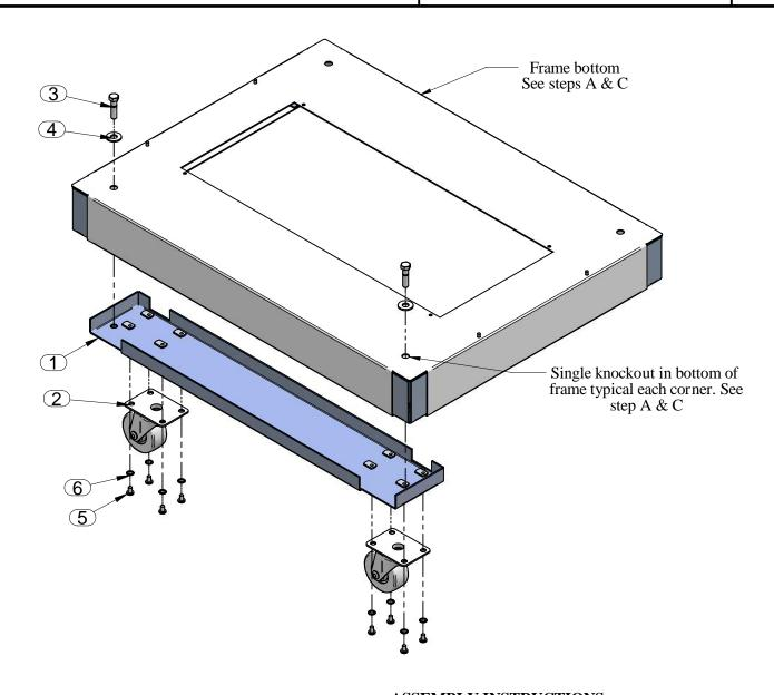
Note: Assembly shown is typical on each side
