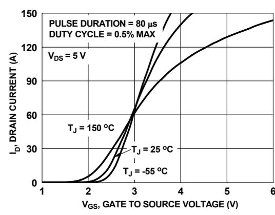
Figure 5. Transfer Characteristics
