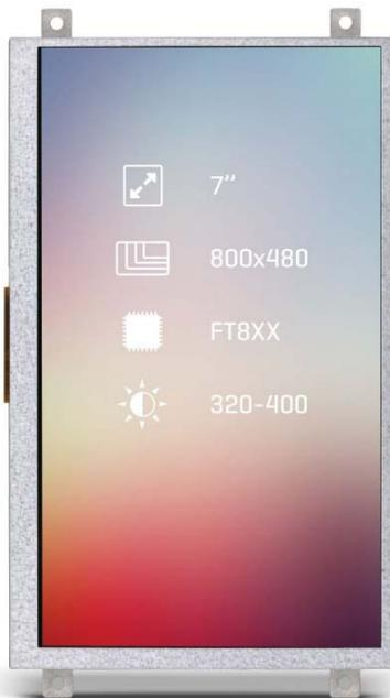
The **800x480px** screen is driven by an **FT812** graphic controller which is supported in Visual TFT, the GUI design tool for rapid development of user interfaces.
