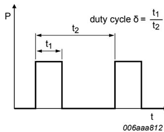
Fig. 18. Duty cycle definition
