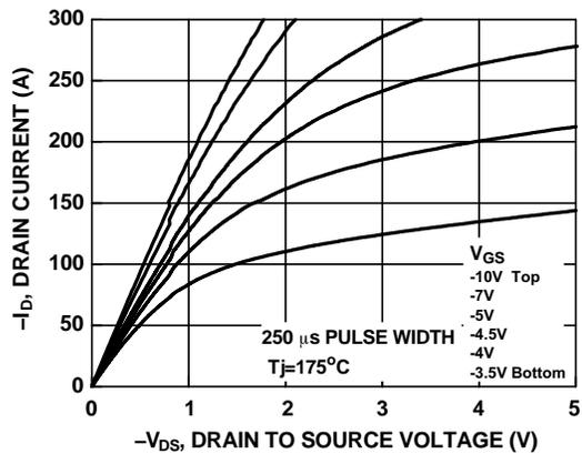
Figure 10. Saturation Characteristics
