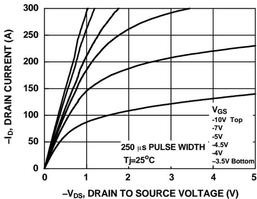
Figure 9. Saturation Characteristics
