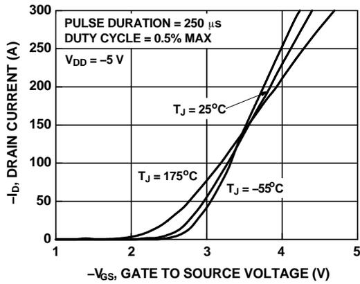
Figure 7. Transfer Characteristics
