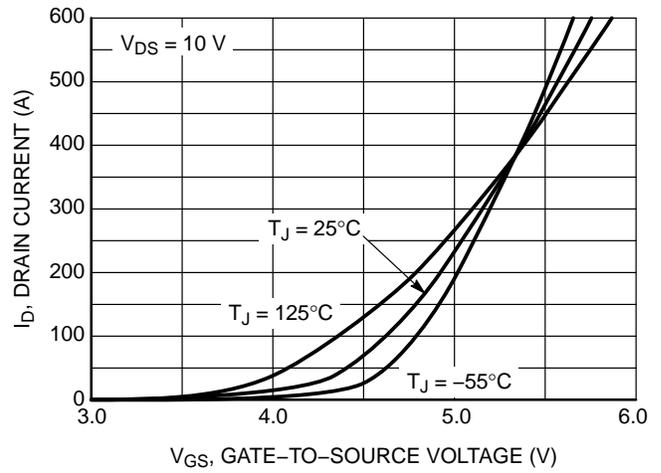
Figure 2. Transfer Characteristics
