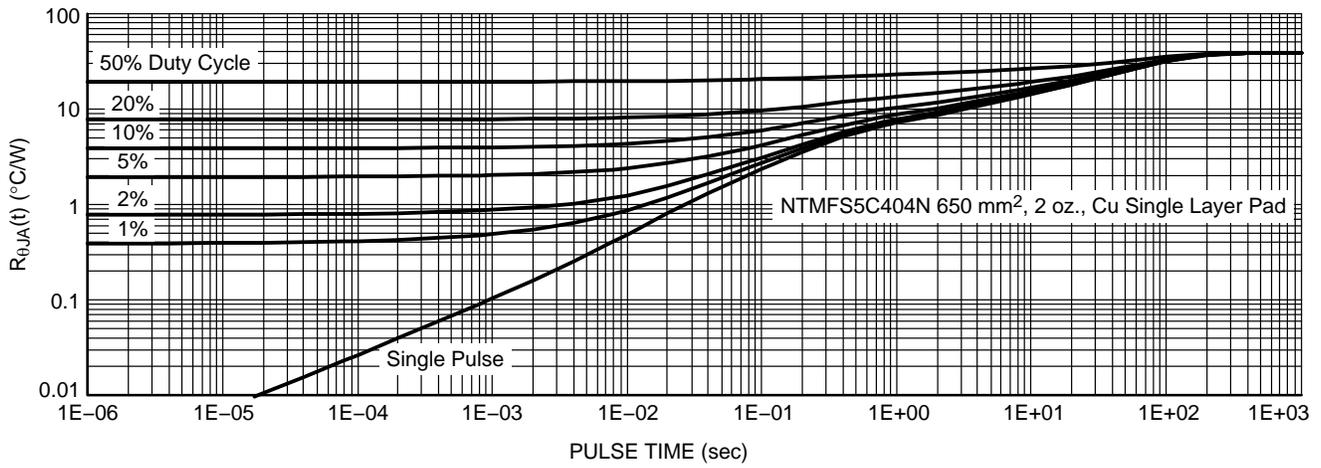
Figure 13. Thermal Characteristics
