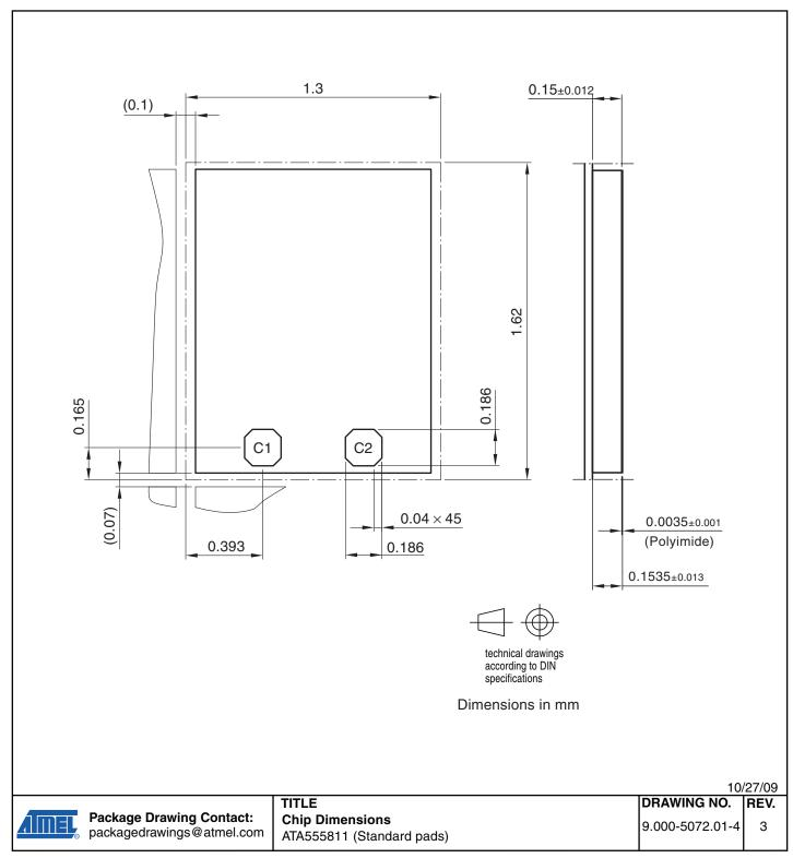
Figure 10-4. Chip Dimensions ATA555811 Standard Pads
