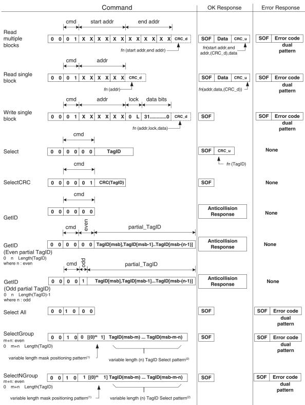
Note: 1. The leftmost position of the TagID select mask is determined by m '0' bits followed by a single '1' bit. These bit positions can be regarded as don't care bit positions.
