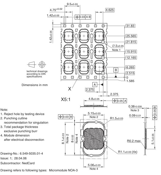
Figure 10-10. Shipping Reel for NOA3 Micromodule
