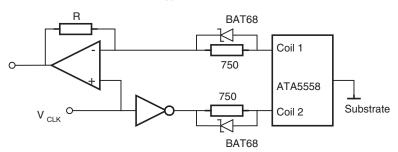
Figure 9-1. Measurement Setup for V<sub>mod</sub>
